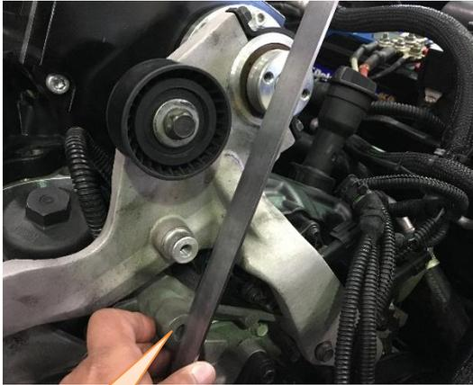
Align steel rule to the mounting face
